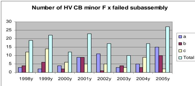
a – Comp. in primary circuit **b** – Comp. in control, auxiliary or monitor. circuit c – Comp. in operating
